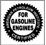
Oils recommended for your vehicle can be identified by looking for the "Starburst" symbol. This symbol indicates that the oil has been certified by the American Petroleum Institute (API). Do not use any oil which does not carry this Starburst symbol.
